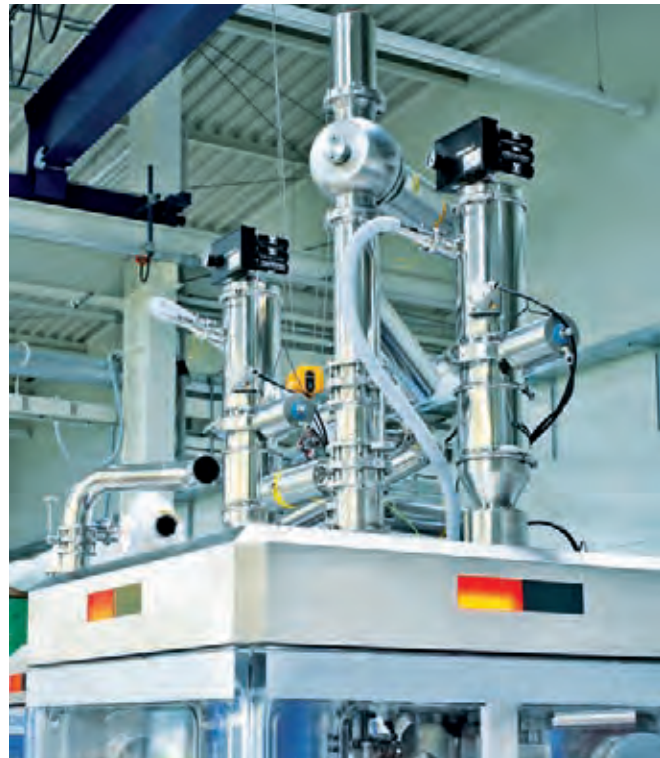
PPC with a WIP function on a tablet press.
