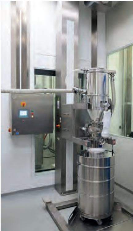
PPC 350VS with rotary valve dosing active substances.
