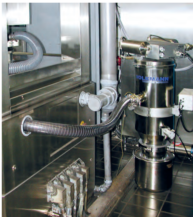
The dust, that occurs inside the tablet press during the pressing, is picked up by an industrial vacuum conveyor
