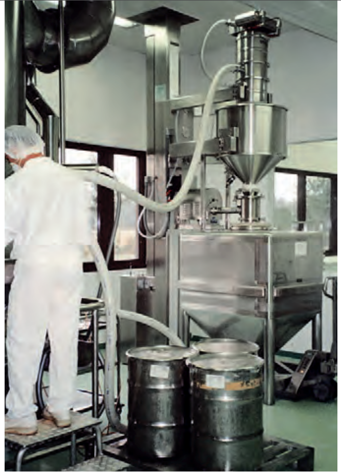
Emptying a dryer with a manual suction lance.
